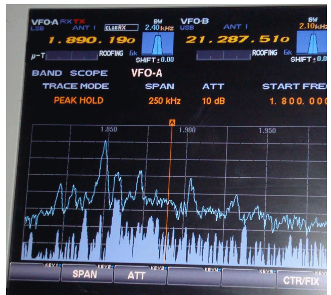
Transmit spectrum trace (lots of noise)
